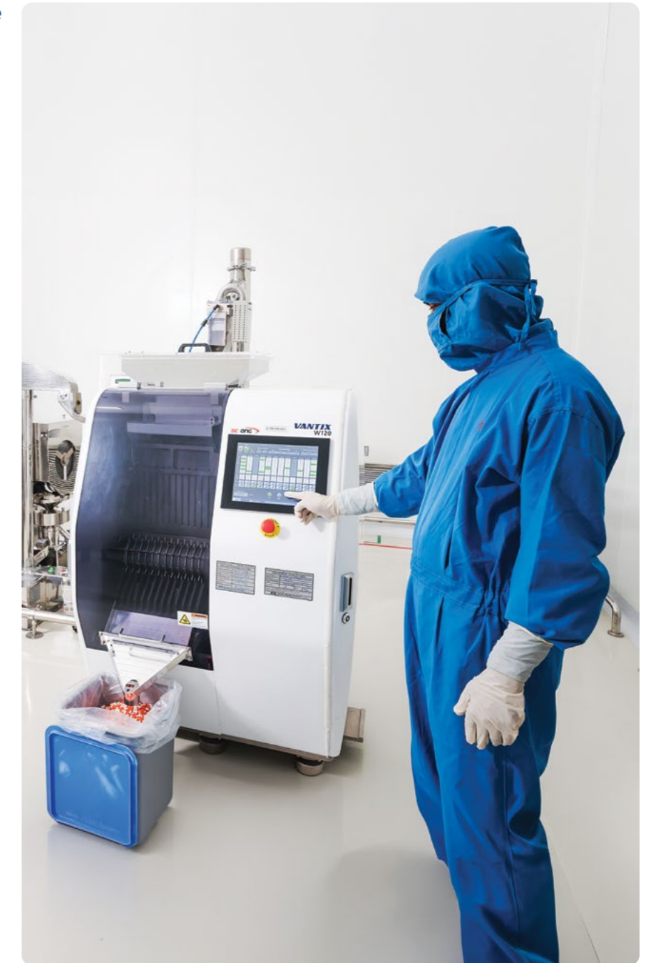
Capsule Filling Line @ Guwahati Facility, Assam
